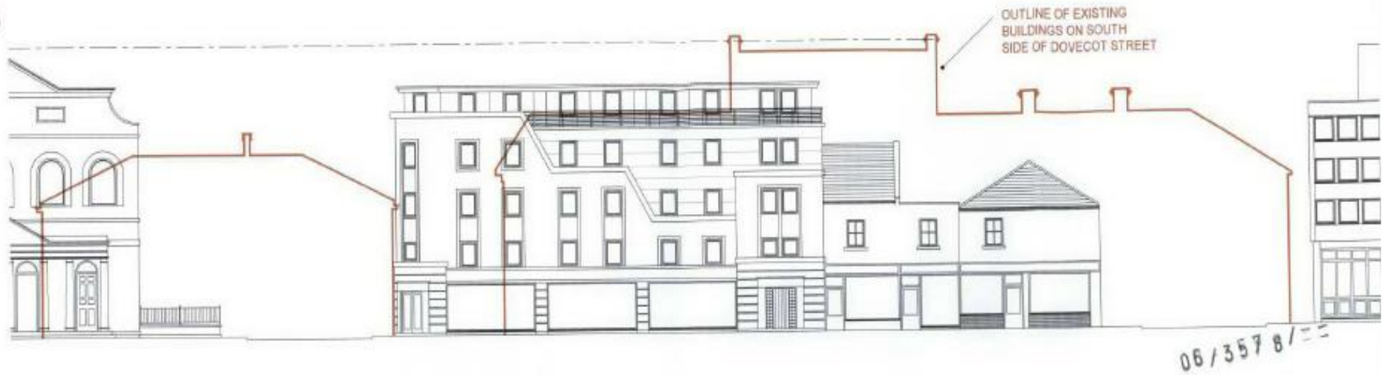
Proposed Street Scene Elevation ( Dovecot Street ) scale 1:200
